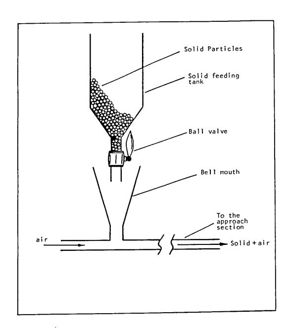
Figure (2.2): Details of solid feeding system.
