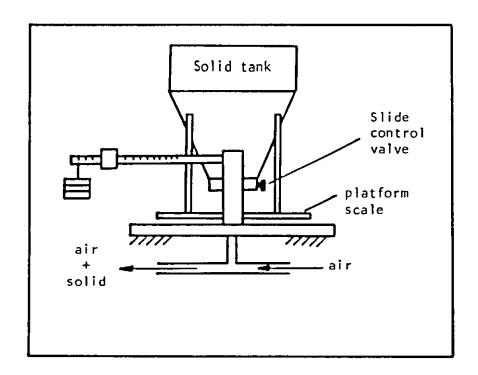
Figure (1.1): Platform scale used in ref. [9].
